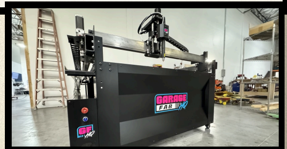
TORCH CARRIAGE: BALL-SCREW Z WITH AUTO TOUCH-OFF AND THC.
