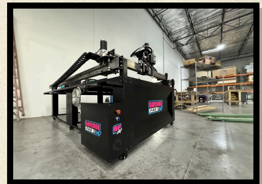
UP TOP: THE RAISED GANTRY, TORCH CARRIAGE AND DRAG CHAIN.
