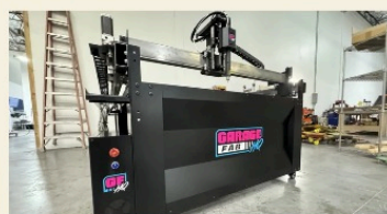
THE CUT THC KEEPS THE GAP DIALED
