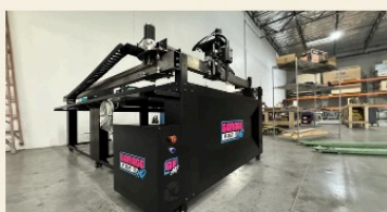
THE GANTRY RAISED FOR 5" OF Z CLEARANCE
